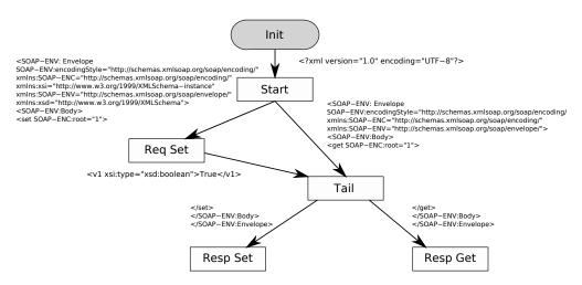
Fig. 1. Finite state machine for get() and set() SOAP messages
