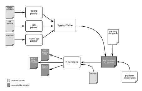
Fig. 2. Compiler block diagram.
