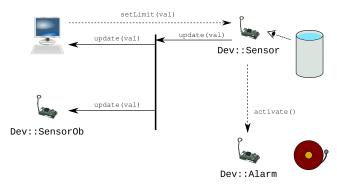
Fig. 3: The tank level controller
