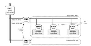
Fig. 2. Example of deployment where different types of EMD are used.
