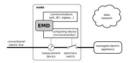
Fig. 1. Block diagram of the general EMD structure.
