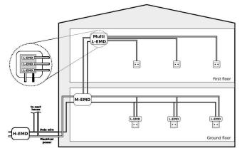
Fig. 3. Example of deployment where different types of EMD are used.
