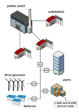
Fig. 5. Example scenario of a power grid where CosGrid devices have been installed.
