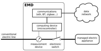
Fig. 2. Block diagram of the general EMD structure.
