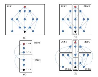
Figure 2. For possible distributions for a semantic tree: (a) single SN, (b) branch partitioning, (c) vertical partitioning with forwards links, and (d) arbitrary combination of both.
