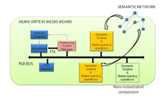
Figure 1. Architecture of the Scone System-on-Chip
