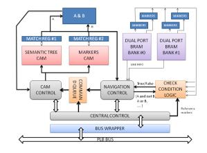
Figure 3. SN internals block diagram
