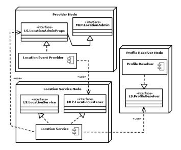
Figure 5. Component diagram of system architecture
