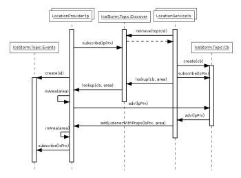
Figure 3. Sequence diagram of the LS discover of LEPs
