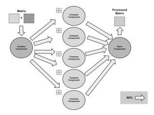
Fig. 8. Logical matrix multiplication architecture
