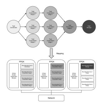
Fig. 7. Application architecture mapping example
