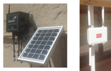
Fig. 2. Civitas pollution monitoring node (left) and service node (right) deployed in the school of computer science
