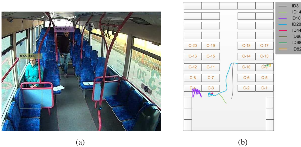
Figure 6: Outputs of the tracker: (a) image with tracker bounding boxes over the person in the scene (b) the corresponding track plots in real-world coordinates
