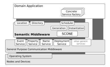
Fig. 1. Overall view of the different modules involved in the proposed middleware architecture
