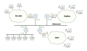
Fig. 4. Prototype IDM topology
