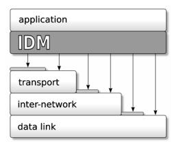
Fig. 2. IDM encapsulation over any layer of the stack
