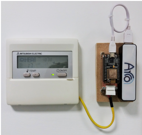
Figure 8. IoT node for temperature control
