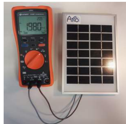
Figure 10. Measurements setup employing the KL-SUN3W PV panel and a Keysight U1242C with data logger functionality.
